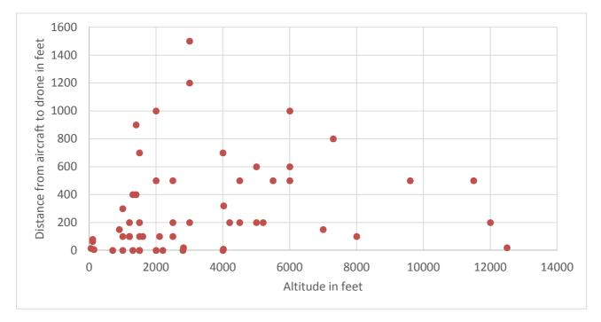
Figure 2 Distribution of RPAS Occurrences - Actual Aircraft Altitude vs Distance to Drone.
